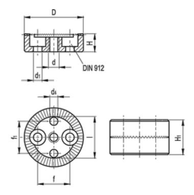
$$\begin{array}{lll} D & = 27 \\ d & = M5 \\ d1 & = 4.3 \\ d4 & H11 & = 4 \\ f & = 15 \\ f1 & = 15 \\ H & +/-0.9 & = 7.5 \\ H1 & = 15 \end{array}$$
